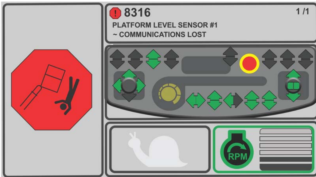
Figure 5-14. Level System DTC Screen
